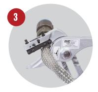
Use the rollover tool to roll over the cutoff tab.
