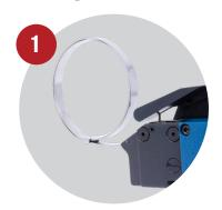
Insert the band loop-side up. Squeeze the blue tensioning handle until the tool locks.
